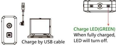
With the DVR powered off, connect USB cable to ③ and the other end of the cable to a computer or a USB charger.
